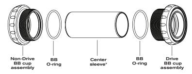
\*Chris King ThreadFit<sup>™</sup> 24 bottom brackets ship with a center sleeve for a 68/73mm bottom bracket shell. For all other bottom bracket shell sizes, the correct center sleeve will be supplied with the approppriate conversion kit.
