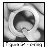
5. Lay a bead of RingDrive<sup>™</sup> lube onto ratchet face of drive ring.
