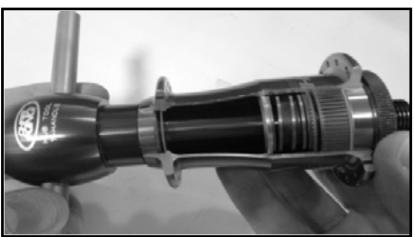
Figure 60 - install non-drive side bearing
