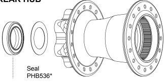
Small Hubshell Bearing PHB700 (Stainless Steel) PHB766 (Ceramic)
