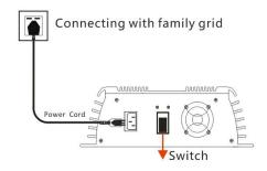
5. Switch on power grid after check for input and output connections are correct and then switch on the Smart Microinverter. The Red/green LED lights up at the same time and then red LED lights off follow on and green LED flash fast, it is means that Smart Microinverter is run for MPPT operation. When green LED long light and it is means that maximum power point lock-in, Smart Micro inverter proper functioning and output steady.
