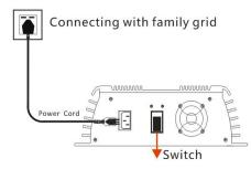
5. Switch on power grid after check for input and output connections are correct and then switch on the Smart Microinverter. The Red/green LED lights up at the same time and then red LED lights off follow on and green LED flash fast, it is means that Smart Microinverter is run for MPPT operation. When green LED long light and it is means that maximum power point lock-in, Smart Micro inverter proper functioning and output steady.
