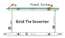
3. Properly connect the positive and negative of solar panel and Smart Microinverter,
