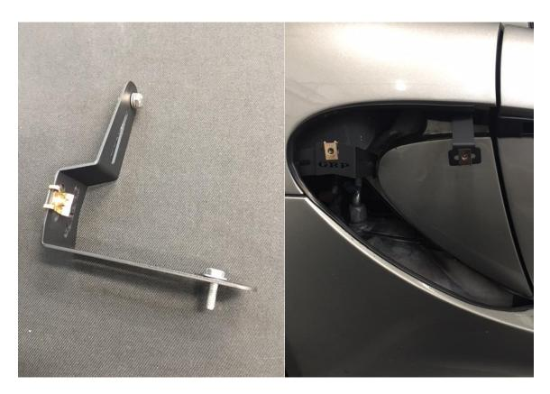
6. Next test fit the Side scoop in place, look closely at the top two hole locations, the outer edge of the carbon vs. the black trim on the clam as well as the bottom edge of the scoop where it meets the bottom rocker panel.
