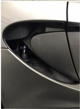
4. Install the appropriate top bracket (driver side or passenger side) assembly into the square opening in the clam tucked under the outer edge just behind the door. This will take some wiggling back and forth to feed the square bracket into the opening, it is sized just right. Once you have the bracket fed in, Lightly tighten the assembly down as shown below.
