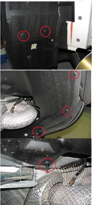
3. Next remove the OEM Plastic side grill. The air intake and snorkle will also need to be removed on the driver's side.
