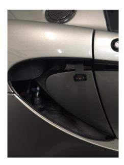
5. Next install the appropriate middle bracket using the oem bolts from the side grill. Be sure to use the two supplied washers on the outside non-slotted hole opening. Not doing so can result in paint DAMAGE! Some cars came with longer bolts than others for this location so it is safe practice to use two washers. Lightly snug the bolts down once in place.
