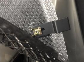
8. With the bottom bracket installed loosely, using a rolling motion hook the bracket inside of the bottom rocker panel and carefully slide/push the scoop up into place. Install the top two outer bolts and washer in the remaining holes in the scoop (those with wide scoops will also need to install the supplied spacers between the scoop and brackets). Double check your fitment, adjust as necessary and tighten up the bolts.
