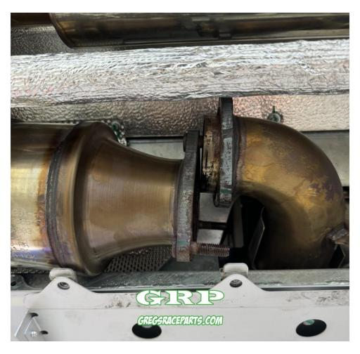
6. Once the flange side is apart you will need to wiggle/work the other end out of the muffler inlet. This side can also be a bit sticky and require some elbow grease. You can use a mallet to aid in popping them loose/apart. We used a mallet and a wood dowel to strike the cat pipe as close to the muffler inlet as possible to help pop it loose then it was easily wiggled/rotated some up and down until it came free.
