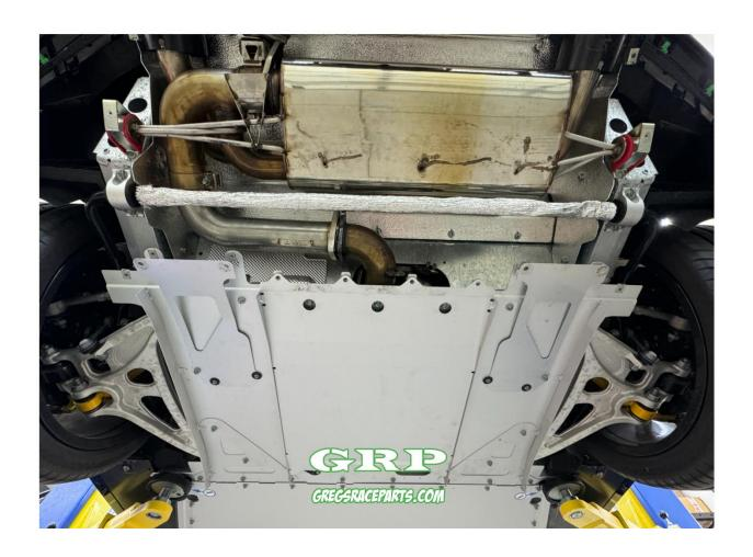
10. Install the other two 15mm hex bolts and nuts and tighten down all three in an even and repetitive manner. These bolts can be torqued to 35-45 ft lbs.
