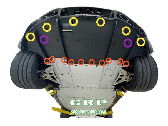
3. Once the diffuser panel is out of the way loosen the 15mm nut circled in yellow on the band clamp between the stock cat pipe and muffler. The clamp is welded and does not spin or move. Then remove the three 16mm nuts circled in red between the cat pipe and mid-pipe flange.
