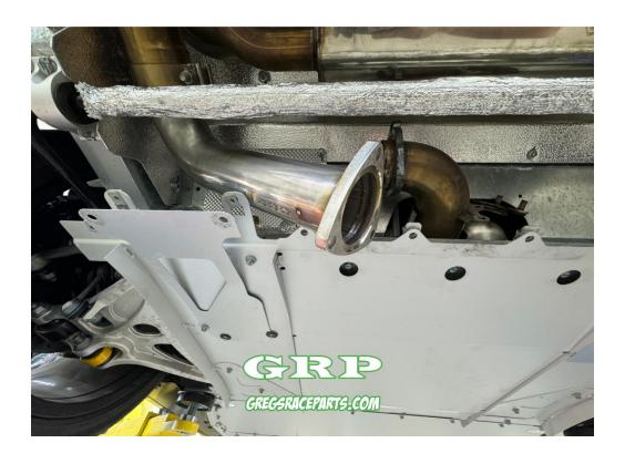
9. Taking care to line up the gasket properly press/squeeze the flanges together and get one of the new supplied 15mm hex bolts and nuts in place. Hand tighten.
