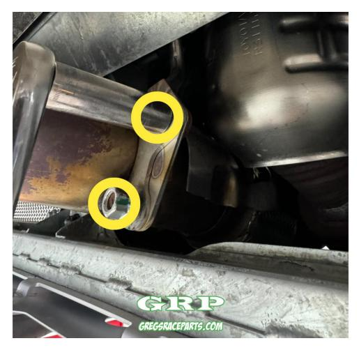
5. Using a little bit of elbow grease you will now need to carefully pry apart the midpipe and original cat pipe until you get the three welded studs to fully disengage from the midpipe. When you loosened the three nuts earlier it should have popped apart slightly already so you can get your pry tool between the flanges and work them apart. Sometimes having two pry tools, a screwdriver handle etc will help a lot here as you can hold it apart with one while you work it apart more with the other.
