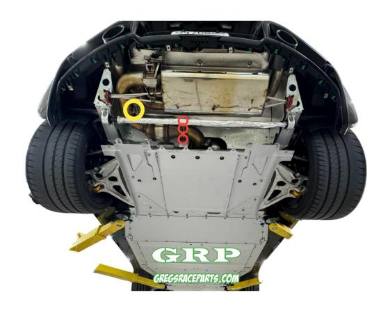
4. Remove the two 15mm nuts circled in yellow at the midpipe exhaust hanger, this is not be 100% needed but opens up more room for movement in the following steps. Push hanger out of the way towards right side of the car.
