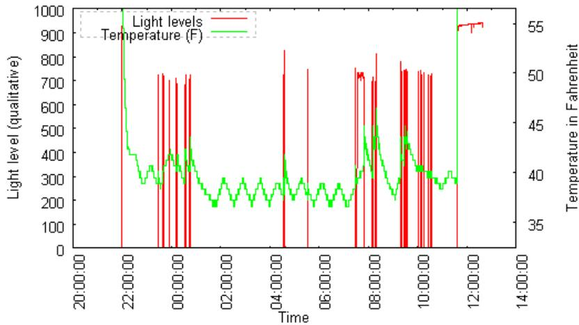
You can see in the middle and end the temp and light levels are very high because the logger was outside the fridge. The green line is the temperature so you can see the temperature slowly rising and then the compressor kicking in every half hour or so. The red lines indicate when the door was opened. This night was a more insomniac one than normal!
