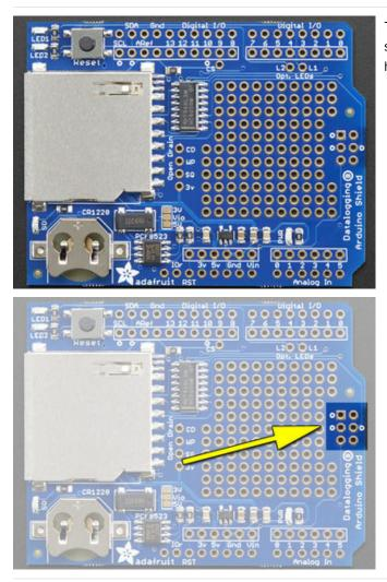
This is the "R3 compatible" Datalogger. Note that it has a smaller prototyping area and that there is a 2x3 SPI header spot on the right
