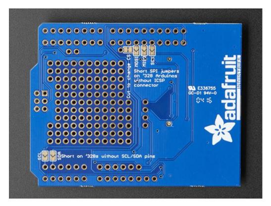
If you are using the shield with a 3.3V logic Arduino, you may want to change the **Vio** jumper. This is what the 10K pullups for I2C are pulled up to. Honestly, the pullups are very weak so if you forget, it's not a big deal. But if you can, cut the small trace between the center pad and 5V and solder the other side so that Vio is connected to 3V
