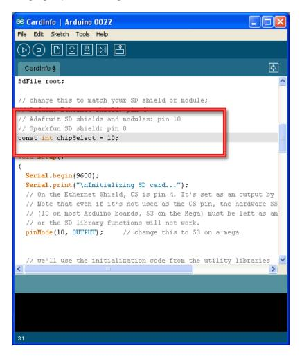
If you have the pre-rev B version of the Datalogger Shield, and you are using a Mega or Leonardo check here for now to adjust the pin setup (https://adafru.it/ref)
