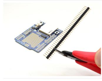
Cut the headers to length: Line the header strip up with the holes on the edge of the shield and cut 4 sections of header strip to fit.
