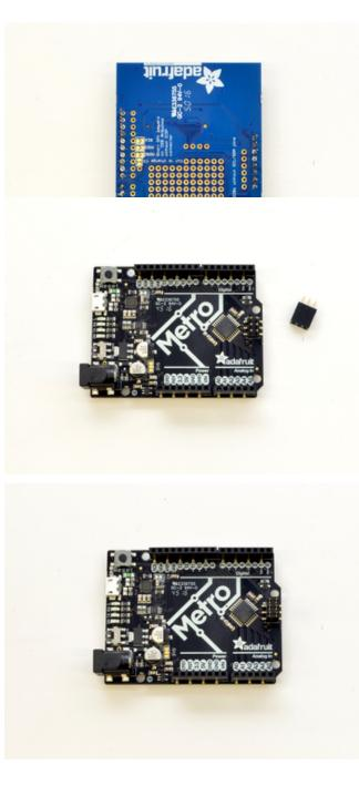
Place the 2x3 female header on to the Arduino/Metro
