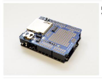
Position the shield: Align the shield with the header pins and press down.
