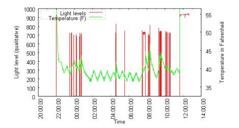
You can see in the middle and end the temp and light levels are very high because the logger was outside the fridge. The green line is the temperature so you can see the temperature slowly rising and then the compressor kicking in every half hour or so. The red lines indicate when the door was opened. This night was a more insominac one than normal!
