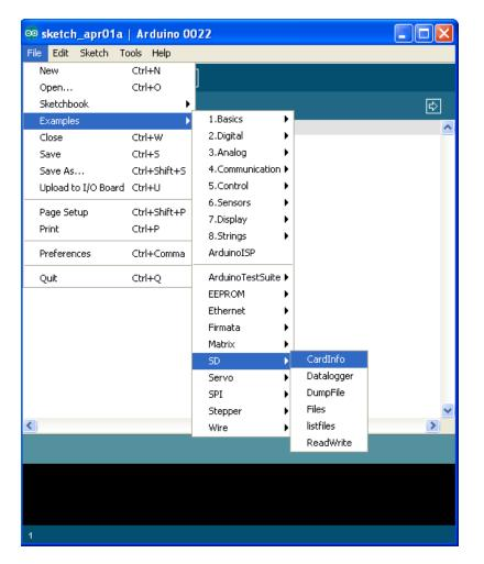
This sketch will not write any data to the card, just tell you if it managed to recognize it, and some information about it. This can be **very** useful when trying to figure out whether an SD card is supported. Before trying out a new card, please try out this sketch! Go to the beginning of the sketch and make sure that the **chipSelect** line is correct, for the datalogger shield we 're using digital pin 10 so change it to 10!
