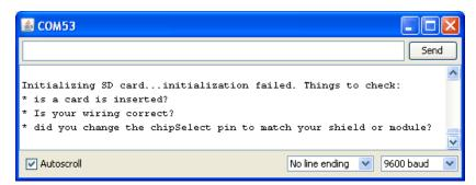
It couldn't even initialize the SD card. This can also happen if there's a soldering error or if the card is really damaged
