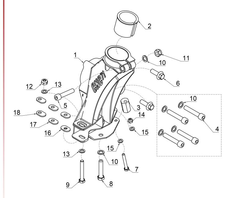
parts 4 and 10 (for hubs assembly) and 6 (caliper) are included into set in separate box.
