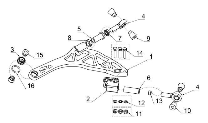
Using an allen key and wrench, loosen the counter bolt. (13)
