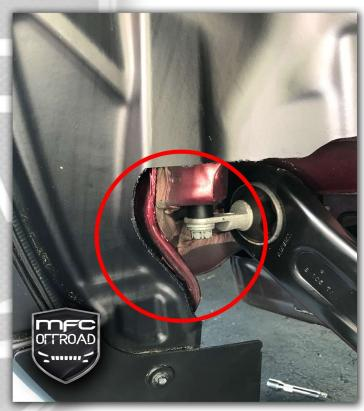
13. Take note of the newly exposed pinch weld. This will be ground down just the same as the front. Grind it so its flat with the trimmed liner. Feel free to go back a full 1/2" - 3/4". You can then hit it with some spray to protect it from the elements as you did with the fronts. The pinch weld modification is now complete!
