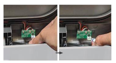
7. Use screwdriver to slide tabs toward the center. Make sure both tabs have been moved to their end-most positions.
