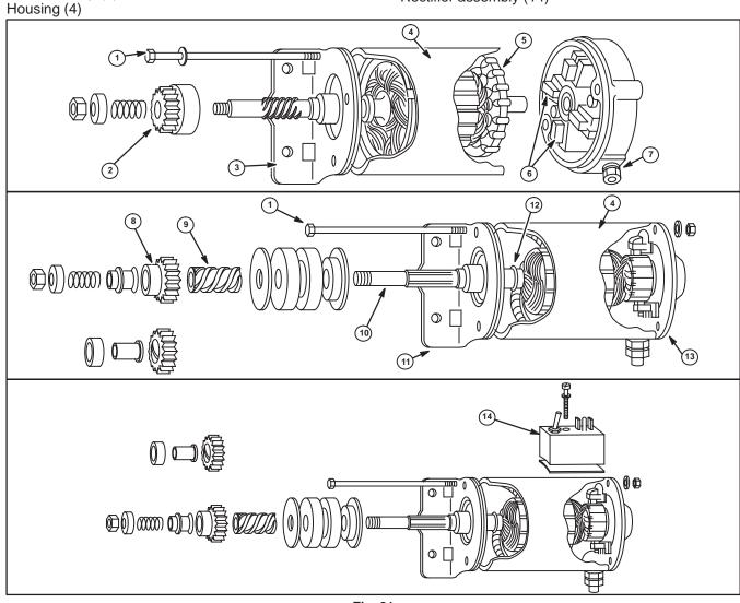
Disassemble Starter Motor Drive Exploded Views – Fig. 81
