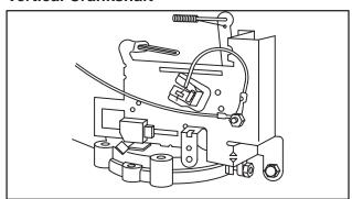
Fig. 6 – 194700, 195700, 196700, 254700, 257700, 258700, 259700, 28A700, 28B700, 28C700, 28D700, 28E700, 28M700, 282700, 283700, 285700, 286700, 289700 with Horizontal Rack & Pinion control for Briggs & Stratton/Walbro LMT Carburetors
