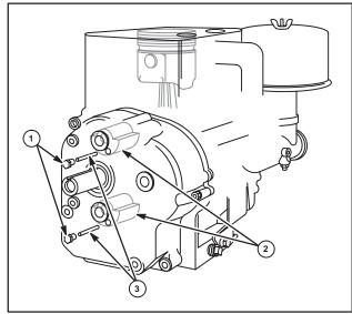
Fig. 7 - Timing Counterbalance Gears
