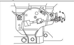
Fig. 51 - Manual Choke, Remote Control, Governed Idle
