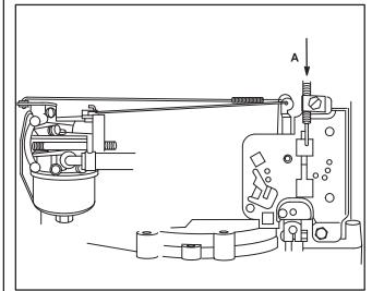
Move as shown (A) to increase speed, Figs. 110-111. Fig. 110
