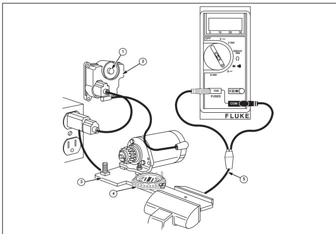
3. Connect AC shunt (5) to a 120 volt outlet.
