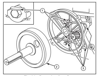
Fig. 34 – Removing Gear Case
