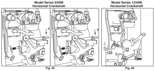
Fig. 45 – Move lever (A) as indicated to increase speed.
