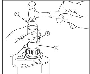
**Disassemble Starter Motor, C-Ring Retainer**
