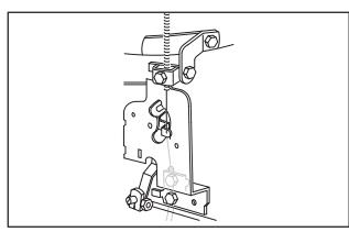
Fig. 10 – Early Style, 170700, 171700, 190700, 191700, Swivel Control Bracket for Briggs & Stratton One Piece Flo-Jet Carburetors
