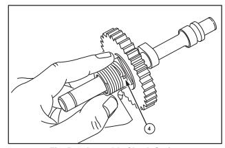
Fig. 58 – Assemble Clutch Spring
