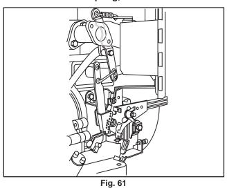
Model Series 176400, 19B400, 19E400, 19F400, 19G400, 192400, 196400, 197400 with Bell Crank Controls and Two Springs, Horizontal Crankshaft
