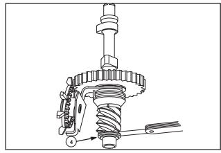
Fig. 55 - Check Cam Gear
