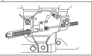
Fig. 53 - Vehicle Controls, Throttle Return
