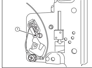
3. Hold throttle in closed position with finger, adjust idle speed screw (1) to 1550 RPM. 4. Release throttle.
