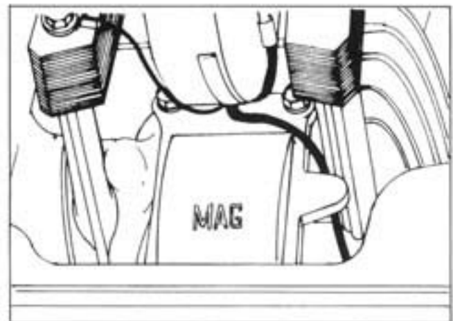
Fig. 21 — Primary Wire Routing
