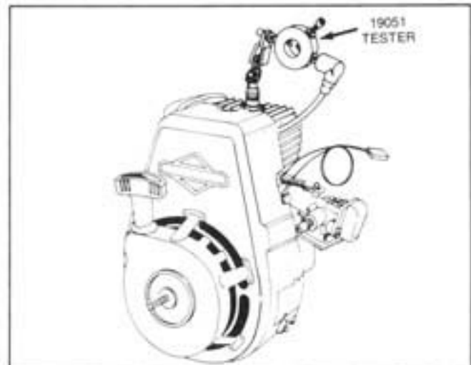
Fig. 2 — Check for Missing — Spark or Fuel
