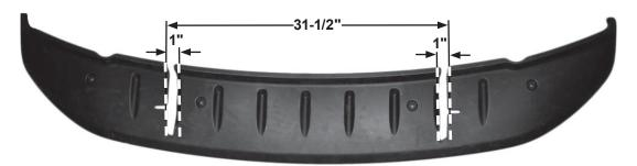
Cut slots in air dam as shown.
