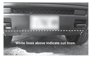
b. Sand and paint sharp edges or add a strip of edge trim to prevent rust.
