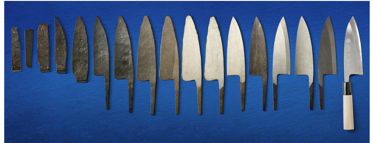
Left to right: 1. Jigane (soft steel) 2. Hagane (hard steel) 3. Initial Forge Weld 4. Forge Weld 5. Initial Shaping 6. Tang Shaping 7. Blade Shaping 8. Blade Thinning 9. Blade Thinning (cont.) 10. Initial Grinding 11. Grinding (cont.) 12. Final Shape 13. Hardening 14. Tempering 15. Finish Grinding 16. Sharpening 17. Handle and Engraving.
