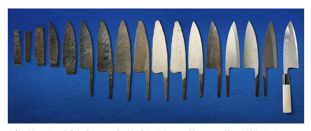
Left to right: 1. Jigane (soft steel) 2. Hagane (hard steel) 3. Initial Forge Weld 4. Forge Weld 5. Initial Shaping 6. Tang Shaping 7. Blade Shaping 8. Blade Thinning 9. Blade Thinning (cont.) 10. Initial Grinding 11. Grinding (cont.) 12. Final Shape 13. Hardening 14. Tempering 15. Finish Grinding 16. Sharpening 17. Handle and Engraving.
