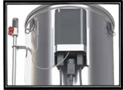
**3.** Attach all plugs and temperature probe connection. Plug the cord from the pump into the pump inlet underneath the control box, do the same for the plug coming from the boiler. The plug exiting the pump is the pump plug, the plug exiting the boiler base is the heating element plug. **NOTE:** You are likely to want to lift the unit up to insert this, but remember it is best to brew with the Grainfather on the floor due to heavy lifting later on.
