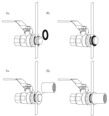
Fill with water to leak test. If leaking from the O-rings next to the kettle wall, ensure that the O-rings are properly seated and try slightly tightening the locknut. If leaking from the ball valve, remove and apply more thread tape.
