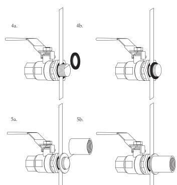
Fill with water to leak test. If leaking from the O-rings next to the cooler wall, ensure that the O-rings are properly seated and try slightly tightening the locknut. If leaking from the ball valve, remove and apply more thread tape.
