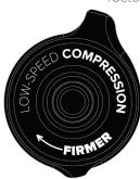
As you turn the dial clockwise, you are adding compression damping or slowing the forks compression stroke. It is an adjustment that is subtle, and often overlooked, but can make a big difference in how your fork performs. Aggressive riders tend to like more compression damping because it provides a firmer, more positive feel. Comfort oriented, less aggressive riders tend to like less because
