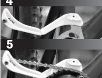
Unthread the upper guide bolt from the captive slider nut, pull it halfway through the upper guide, and swing the upper guide open.
