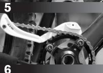
Install the crankset and chain. Close the upper guide and reinstall the upper guide bolt. Tighten the upper guide bolt to 1.2-1.3 Nm. The backplate features laser etching to assist in the vertical positioning of the guide. There should be roughly 3mm of space between the chain and the ceiling of the upper guide.
