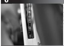
Check that the alignment of the guide is correct. The chain should be centered in the upper guide in the middle range of the cassette. There should be little or no contact between the chain and upper guide while in the smallest or largest cogs of the cassette. Refine this spacing using the included .5mm and 1mm washers if necessary.\*
