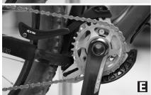
Install the crankset and chain (FIG. E). Close the upper guide and reinstall the upper guide bolt. Tighten the upper guide bolt to 1.2-1.3 Nm (FIG. F). The backplate features laser etching to assist in the vertical positioning of the guide. There should be roughly 3mm of space between the chain and the ceiling of the upper guide.
