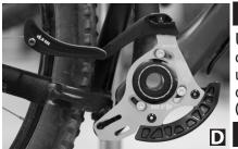
Unthread the upper guide bolt from the captive slider nut, pull it halfway through the upper guide, and swing the upper guide open. Remove the lower guide assembly (FIG. D).
