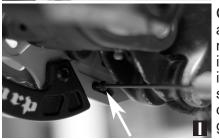
Check that all fasteners have been appropriately tightened and that there is no unwanted rubbing or contact anywhere in the assembly. On full-suspension installations, remove the air or coil from the shock and fully cycle the suspension to be certain. Check the functionality of the of the guide in a safe environment.
