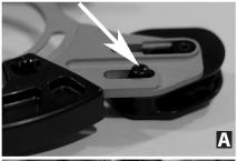
From the backside of the guide, remove the 3mm bolt threaded into the peg of the lower guide (FIG. A).
