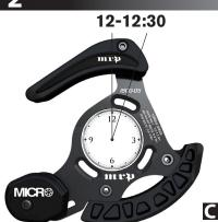
Adjust the guide so that the upper guide bolt is located between 12:00 and 12:30 relative to the center of the BB (FIG. C). Once there, tighten the ISCG screws to 8-9 Nm or BB cup (for BB-mount guides) to its recommended torque.
