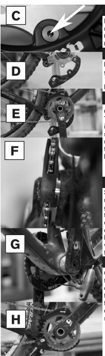
From the back of the guide, use a 4mm allen key to remove the rearward skid bold from the lower portion (FIG. C). Swing the lower portion of the guide down (FIG. D).
