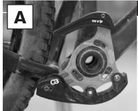
Using a 4mm allen key fasten the guide to the frame's threaded tabs using the included ISCG screws (FIG. A). As needed, install the included 1mm spacers. Typical ISCG spacing (assumes tabs are flush with face of BB shell) is 1mm for 73mm, and 1mm for 83mm shells.\* These spacers always go between the backplate and the frame's threaded tabs. Leave the ISCG screws slightly loose for now.
