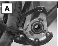
Using a 4mm allen key fasten the guide to the frame's threaded tabs using the included ISCG screws (FIG. A). As needed, install the included 1mm spacers. Typical ISCG spacing (assumes tabs are flush with face of BB shell) is 1mm for 73mm, and 1mm for 83mm shells.\* These spacers always go between the backplate and the frame's threaded tabs. Leave the ISCG screws slightly loose for now.
