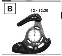
Adjust the guide so that the upper guide bolt is located between 12:00 and 12:30 relative to the center of the BB (FIG. B). Once there, tighten the ISCG screws to 8-9 Nm. Remove the upper guide using a 3mm allen key and 8mm wrench.
