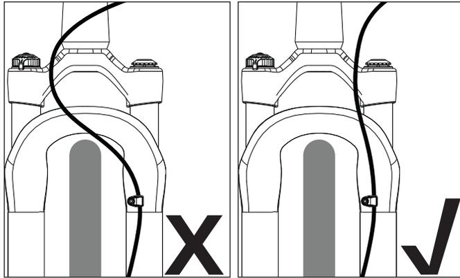
We recommend that your hose not cross the vertical path of your wheel. Failure to trim and route the hose correctly could cause brake hose wear and eventual failure.
