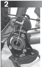
Adjust the guide so that the upper guide bolt is located between 12:00 and 12:30 relative to the center of the BB. Once there, tighten the ISCG screws to 8-9 Nm for alloy backplates, or 5-7 Nm for carbon models.
