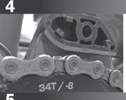
Install the crankset and chain. Reinstall the front of the upper guide and upper guide bolt. Tighten the upper guide bolt to 1.2-1.3 Nm. The backplate features laser etching to assist in the vertical positioning of the guide. There should be roughly 3mm of space between the chain and the ceiling of the upper guide.
