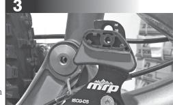
Unthread the upper guide bolt from the captive slider nut and remove the front of the upper guide.
