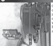
Check that the alignment of the guide is correct. The chain should be centered in the upper guide in the middle range of the cassette. There should be little or no contact between the chain and upper guide while in the smallest or largest cogs of the cassette. Refine this spacing using the included ISCG spacers as needed.
