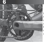
Check that all fasteners have been appropriately tightened and that there is no unwanted rubbing or contact anywhere in the assembly. On full-suspension installations, remove the air or coil from the shock and fully cycle the suspension to be certain. Check the functionality of the of the guide in a safe environment.
