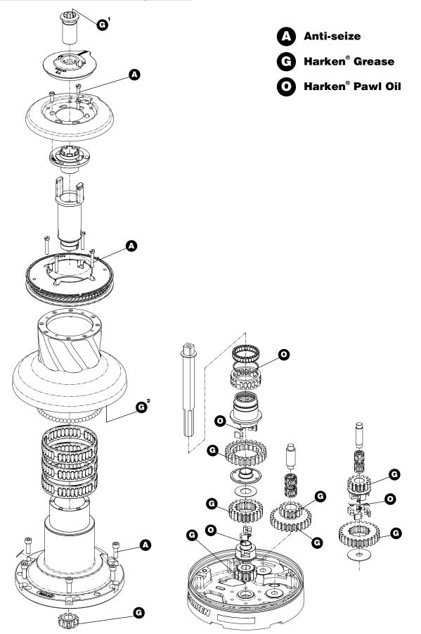
1. Apply Harken® grease on assy socket screw - 2. Apply Harken® grease on drum gear
