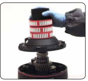
10. Slide out the drum support  $n^\circ 16$
