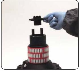
6. Remove the stripper arm housing n°21
