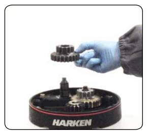
13. Remove the idler and pinion  $n^{\circ}14$
