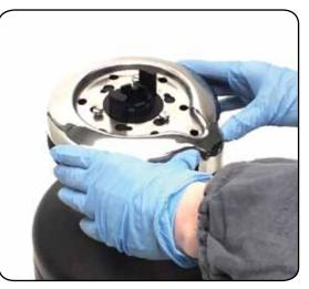
When positioning the stripper arm, align the peeler with it. If the jaws have been disassembled, insert peeler between the two jaws, taking care that the letters TOP on the peeler are facing upwards.
