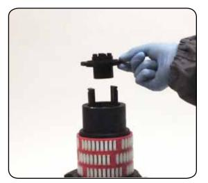
6. Remove the stripper arm housing n°21
