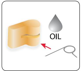
**To assemble the pawls** Correctly position the spring in its housing as shown at left. Hold the spring closed and slide the pawl into its housing. Once in position, check that the pawls can be easily opened and closed with a finger.
