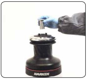
2. Slide off the assy socket  $n^\circ 30$  and the cover  $n^\circ 29$
