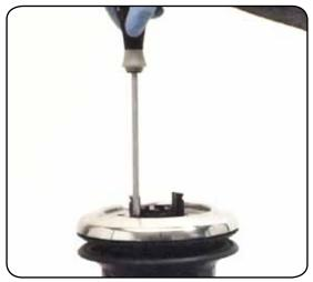
3. Unscrew the three screws n°28 (~4Nm/35 in-lb)
