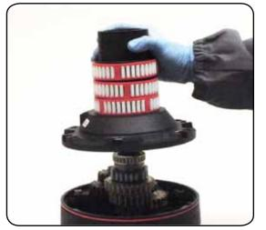
10. Remove the drum support  $n^\circ 16$
