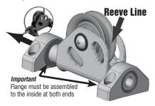
To achieve maximum working load use four (4) screws with backing plates, washers and locknuts. Use only A4 (316) or A2 (18-8) fasteners in the size listed in chart on the reverse side. Ensure deck strength is equal to block strength.
