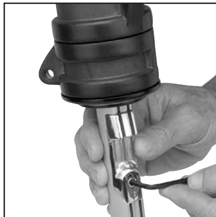
Loosen screw one revolution only .
