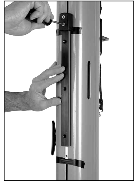
3. Thread a 8 x 40 mm screw through endstop, track, and into endstop slug.
