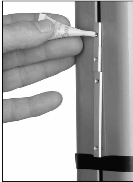
2. One drop blue Loctite® adhesive into each connector slug hole.
