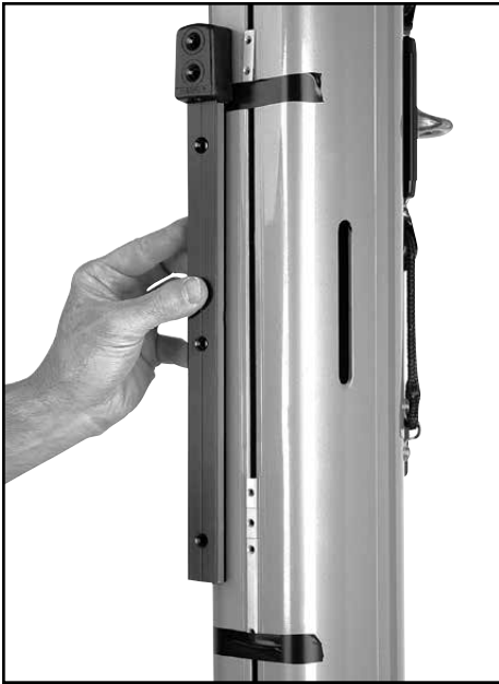
1. Slip top track slugs into mast groove. Use 51 mm (2") mounting slug for top stop.
