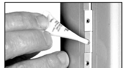
6. Slide 19 mounting slugs and connector slug into mast groove.
