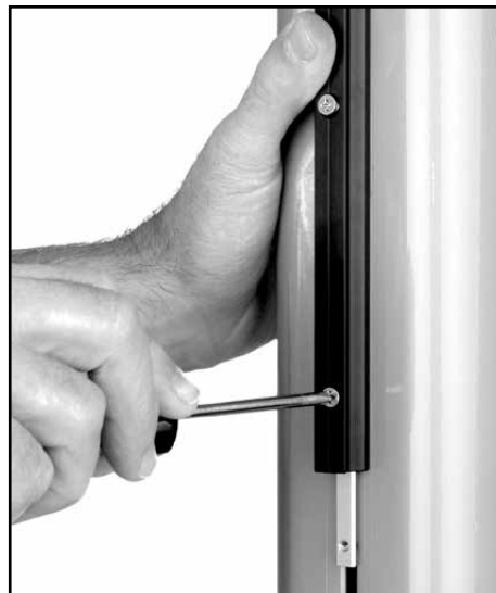
5. Loosen top screw. Slide top track up and position next 2.08 m (6'9 15/16") track.
