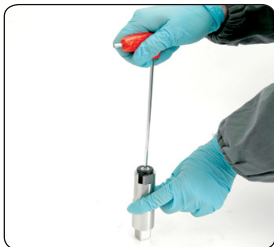
Unscrew the screw n°13 and remove the washer n°12 ( \approx 4\text{Nm}/35\text{ in-lb} )
