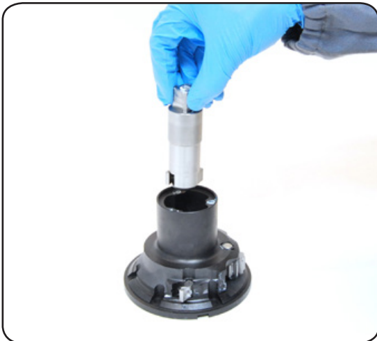
8. Slide out the central shaft n°14
