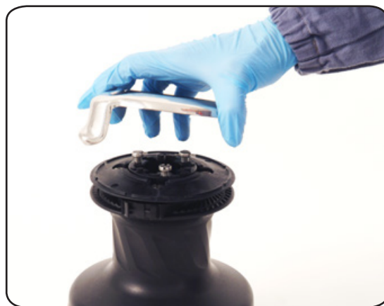
4. Remove the self-tailing arm n°18 by rotating and lifting it.
