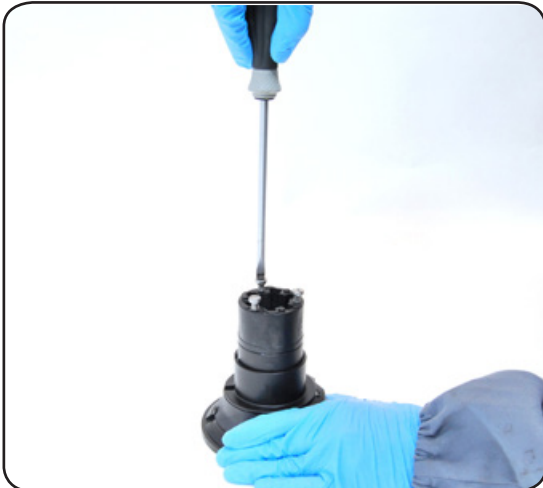
6. Completely unscrew the three screws n°17
