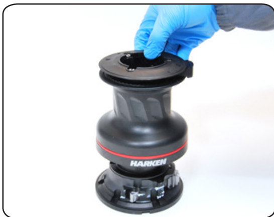
5. Lift off the drum n°7
