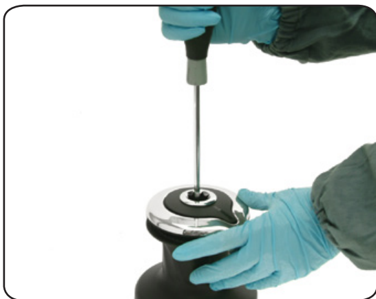
1. Unscrew the central screw ( \approx 2\text{Nm}/18\text{ in-lb} )
