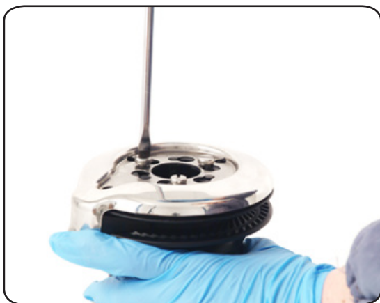
3. Unscrew the three screws n°17 ( \approx 4\text{Nm}/35\text{ in-lb} )
