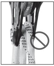
If Loup is stacked (one strand on top of the other) even a small amount, line can push outward and break sideplate.
