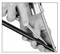
Cut, splay, and snap tube into place.
