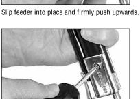
Coat screw with blue Loctite® and tighten. If screw does not thread, check alignment.
