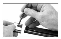
**Tip:** Trim cap holes are different diameters. Make sure 5 mm (3/16") drill bit fits through hole and foil-side grooves face up.
