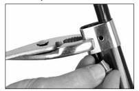
Place trim cap on foil so slot is aft, with large hole on starboard. Squeeze together with pliers. Put blue Loctite® in barrel nut. Install two-piece screw and barrel nut with Phillips screwdriver.
