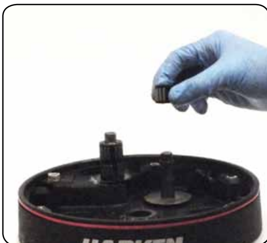
17. Remove the roller bearing n°12
