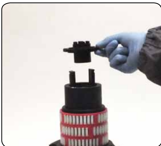
6. Remove the stripper arm housing n°21
