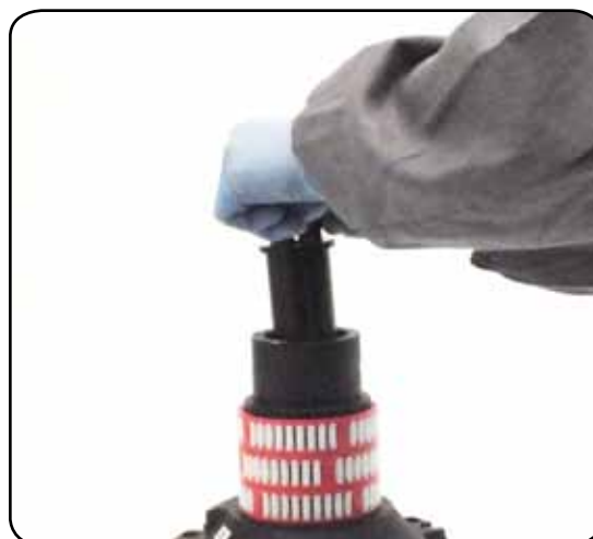
7. Slide out the assy clutch n°37
