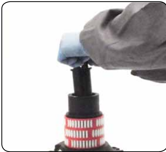
7. Slide out the assy clutch n°37
