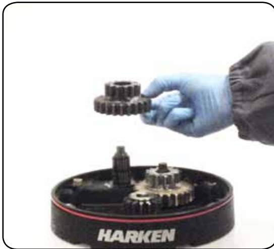
13. Remove the idler and pinion n°14
