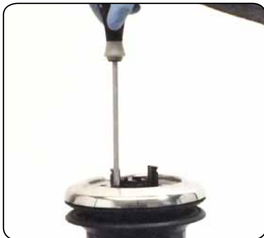
3. Unscrew the three screws n°28 (🔧 4Nm/35 in-lb)
