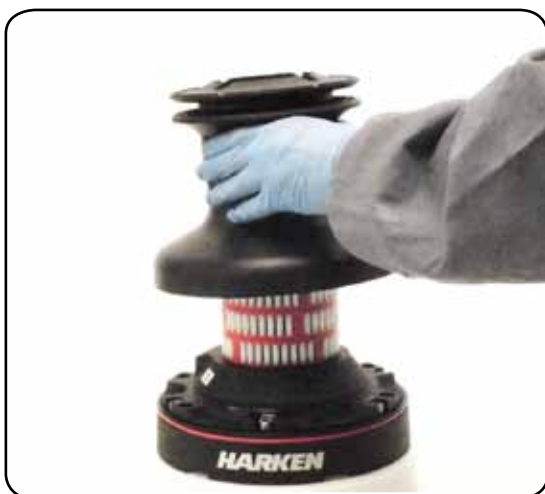
5. Lift off the drum n°24
