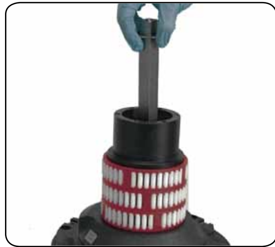
8. Slide out the central shaft n°19
