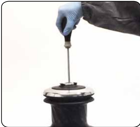
1. Unscrew the central screw (🔧 2Nm/18 in-lb)
