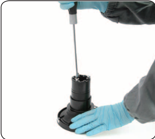
6. Completely unscrew the three screws n°18
