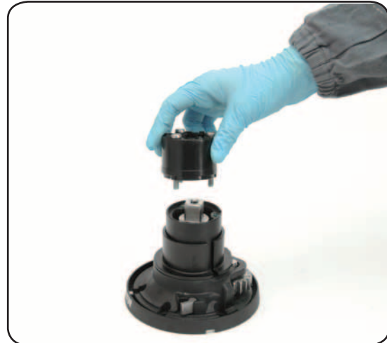
7. Remove the self-tailing arm support n°12 and slide out the bushing
