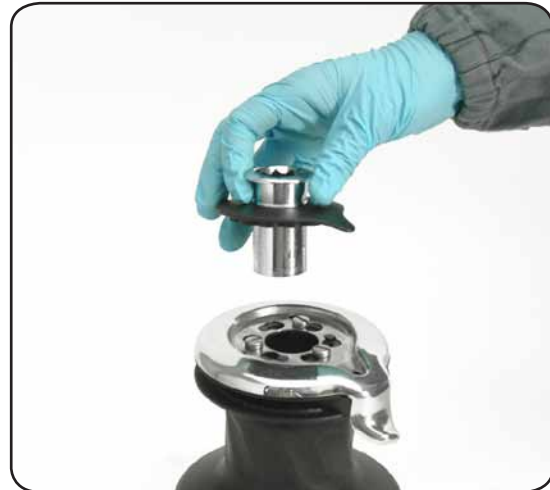
2. Slide off the assy socket n°20 and the cover n°19
