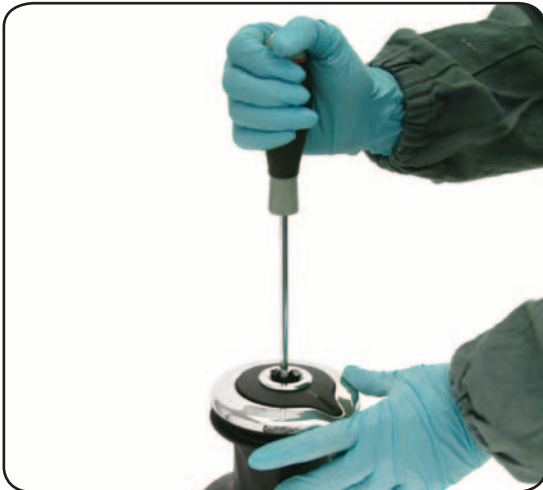
1. Unscrew the central screw ( \approx 2\text{Nm}/18\text{ in-lb} )
