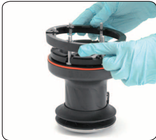
4. Reposition the skirt n°2 in its housing
