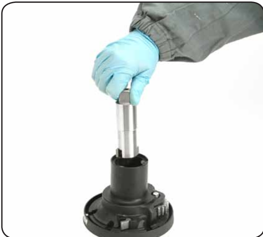
8. Slide out the central shaft n°7
