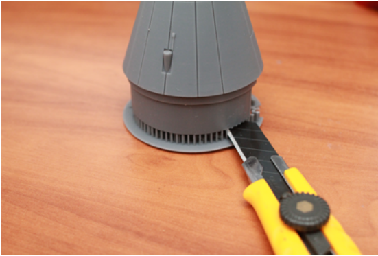
3. Continue by removing the rest of the thinner supports
