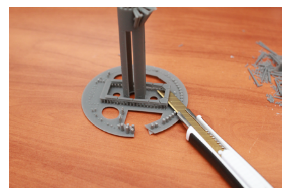
8. Cut off the door frame from the base with a sharp knife
