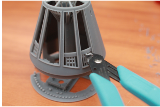
4. Carefully remove the window frame supports on the sides by using a pair of sharp sidecutters
