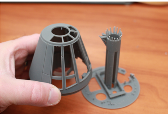
7. You should be able to separate your nosecone from the base and the support structure now
