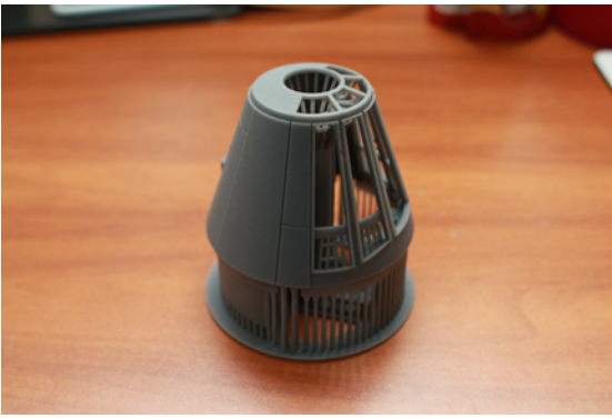
1. Removing supports from the nosecone.
