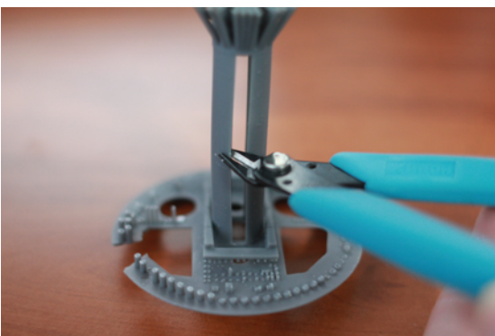
9. Cut the support column in half to be able to remove the door frame
