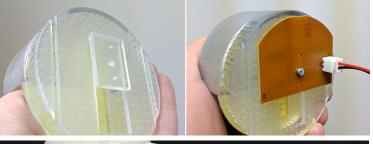
Glue in the adapter for the stock light board to the back of the clear insert.
