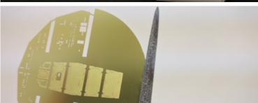
Sand off the support marks on the photo-etched parts with a file. Dry fit the photo-etched sheet for the back wall to the inside wall of the clear insert. Ensure the bottom part of the photo-etched wall is not sticking out of the insert. If it is, sand it with a fine file.
