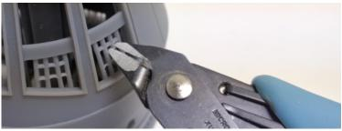
Cut off the supports using a pair of side cutters and an X-Acto knife. Sand off the support marks with a file. Be careful when cutting off the supports from a fragile parts like steering gears.
