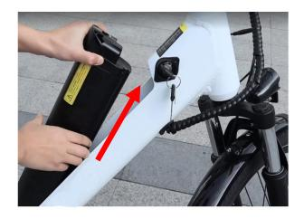
Gently lift the battery from the battery compartment by sliding upward.
