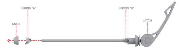
Step 4: Locate the side of the front wheel with the disc. Insert the end of the quick release axle through the hole in the center of the wheel on the side OPPOSITE the disc and push it through to the disc side.
