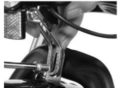
Step 4: Align the fender "U" brace arms to the tabs on the rear side of the front fork
