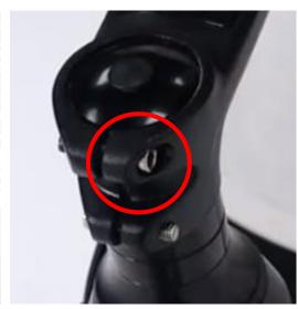
Step 4: Connect the two harness connections.
