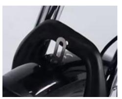
Step 3: Move headlight into place and use the screw to attach the headlight and fender.
