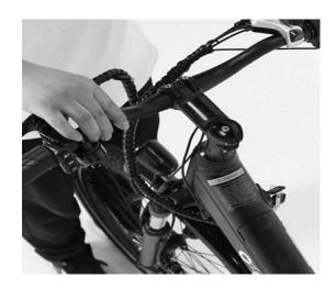
Step 2: Tighten the top screw. When you are finished tightening the screw, add the small rubber cap.
