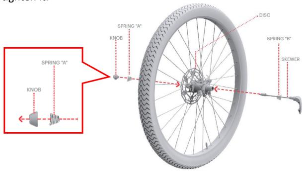
Step 7: Position the front wheel in between the front fork so that the disc side of the wheel is on the side of the fork with the brake components.
