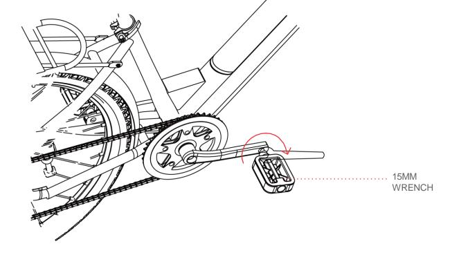
Step 3: Finish inserting and then tightening the spindle into the crank arm by turning it clockwise with the 15 mm wrench or 15mm wrench tip of the multi-tool.
