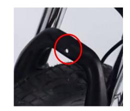
Step 2: Slide front fender through the front fork and over the tire until the tab on the fender meets the fork.
