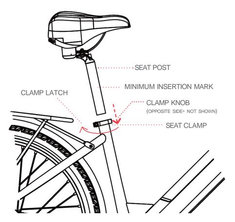
Step 4: To lock the seat in place, close the latch on the seat clamp.
