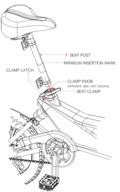
Step 4: To lock the seat in place, close the latch on the seat clamp.
