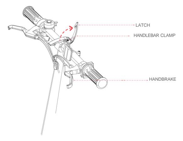
Step 2: Rotate the handlebar forward or backward to reposition it.
