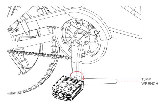
Step 3: Finish inserting and then tightening the spindle into the crank arm by turning it clockwise with the 15 mm wrench or 15mm wrench tip of the multi-tool.
