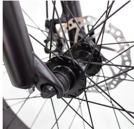
**When properly installed**, the front wheel should be fully seated and centered in the dropouts of the front fork, the brake rotor should be in between the brake pads in the brake caliper, and the quick release lever should be fully and properly secured. Ensure the front wheel and quick release lever are properly secured before moving on to the next step.
