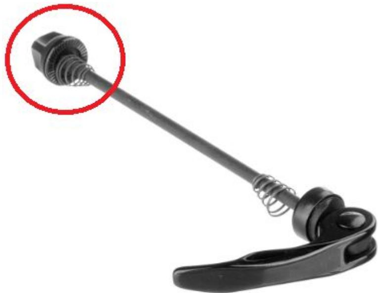
**Install the skewer into the front wheel axle** from the brake rotor side. Reinstall the cone spring so it points toward the wheel hub then thread the thumb nut onto the skewer only a couple turns, leaving room for the fork dropouts. Make sure the lever is open and carefully lower the fork onto the axle and brake caliper as shown below
