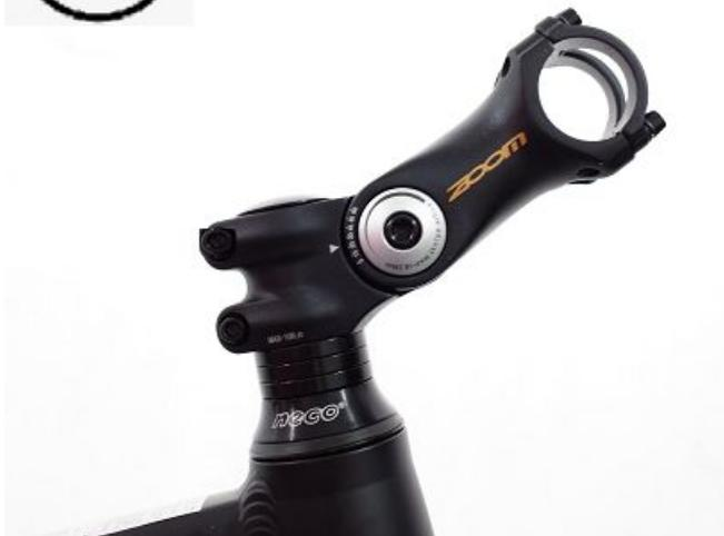
**Step 2:** Loosen the bolt below ( in red circle) using an allen key and then adjust the handlebar stem height to the desired position
