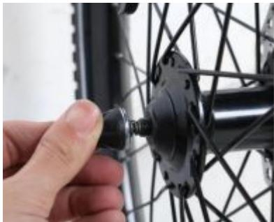
When there is enough resistance to hold the quick release lever in line with the axle, close the lever using the palm of your hand without touching the brake rotor as shown below
