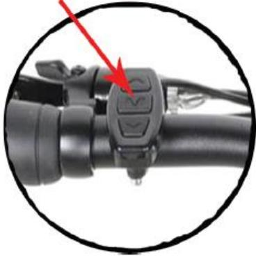
3) Turn on the Headlight/Taillight press and hold the UP arrow for 3 seconds
