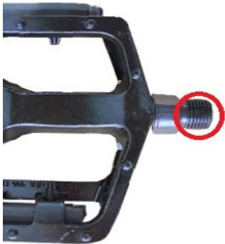
**The right pedal (1) is threaded so that it is tightened by turning clockwise.** Carefully thread the right pedal onto the crank on the right side of the bike slowly and by hand. Do not cross thread or damage the threads and make sure to tighten the pedal with wrench provided
