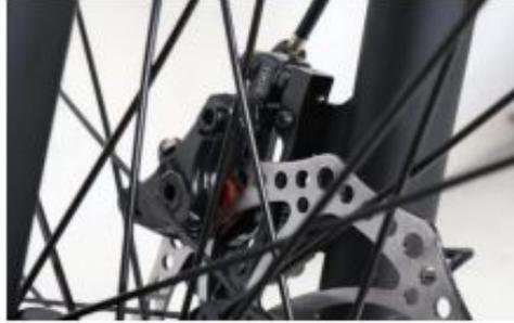
**Fully seat the skewer in the fork dropouts** (and the brake rotor in the caliper) and add tension to the lever by turning the thumbnut, as shown below
