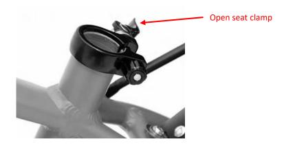
Step 2: Insert the seat post into the seat stem and close the seat clamp.
