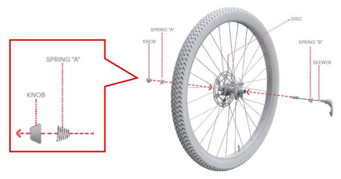
Step 7: Position the front wheel in between the front fork so that the disc side of the wheel is on the side of the fork with the brake components.
