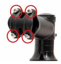
Step 3: Raise the handlebar into place and adjust it to the desired angle
