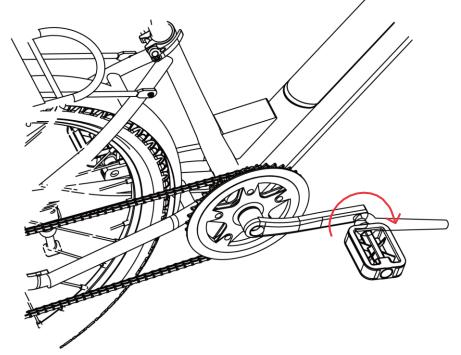
Step 3: Finish inserting and then tightening the spindle into the crank arm by turning it CLOCKWISE
