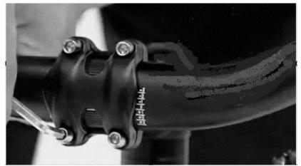
Step 5: After the handlebars are installed, make sure they are aligned with the front tire and carefully tighten the top screw under the rubber cover and the pinch bolts on each side of the stem.
