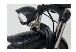
Step 5: Align the fender bracket to the tabs on the fork and tighten the previously removed screws with an Allen key.
