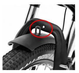
Step 4: Position the headlight bracket between the fork and fender tab. Insert screw that was previously removed and tighten. Adjust the headlight into the proper position.
