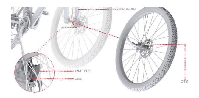
Step 9: When the wheel is centered and in place, tighten the knob on the axle by turning it clockwise. Close the latch on the quick release axle.
