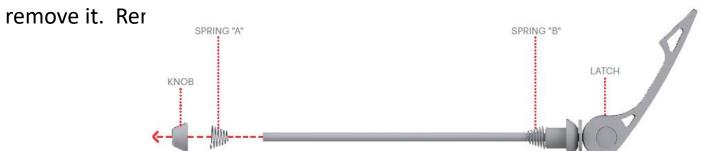
Step 4: Locate the side of the front wheel with the disc. Insert the end of the quick release axle through the hole in the center of the wheel on the side OPPOSITE the disc and push it through to the disc side.
