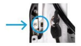
Unlocked-locking pin not protruding through frame
