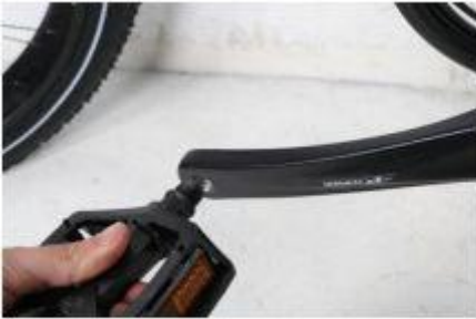
Right Pedal On The Same Side As The Chain
