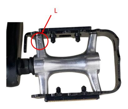
Step 3: Finish inserting and then tightening the spindle into the crank arm by turning it clockwise
