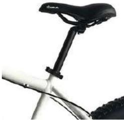
Open the release handle found on the frame of the bike. Then insert the seat tube into the frame. (as seen in the picture to the left)
