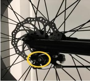
If you feel that your brakes are too tight, turn the silver knob clockwise (clockwise is to the right) and now try to see how the braking of the bike wheel feels. Turning the silver disc clockwise will loosen the brakes, as where turning the silver knob counter-clockwise will tighten the brakes.
