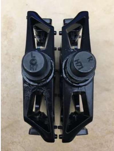
Once you have determined the Right and Left peddles, now twist the pedals toward the front of the bike until they are securely fastened. Please see picture below for how the pedals should look after securely fastened.
