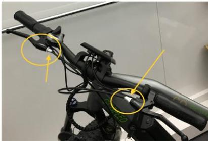
If the brakes still don't feel secure, tighten the silver knobs on the handlebars by the hand brakes. This will tighten the brakes.
