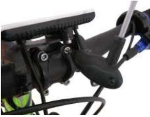
Ensure that all screws on handlebar are securely tightened and in the correct position. You can find the screws to the handlebar behind the LCD monitor on the handlebar of the bike.
