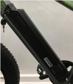
When you put the battery back on the bike frame, put the bottom right of the battery in place first, then align the top of the battery so that the battery is fully secure and connected. Then lock the battery. To lock the battery just turn the key into the locking position.
