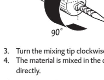
3. Turn the mixing tip clockwise 90° to lock it.
