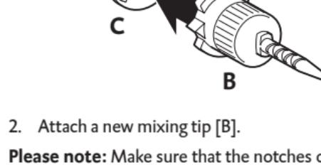
2. Attach a new mixing tip [B].
