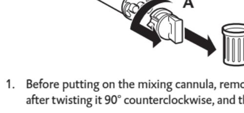
1. Before putting on the mixing cannula, remove the cap [A] or used mixing tip after twisting it 90° counterclockwise, and then discard it.
