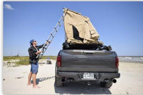
5. Adjust ladder height to achieve a 30 degree angle by depressing the buttons under each rung, starting at the top rung.
