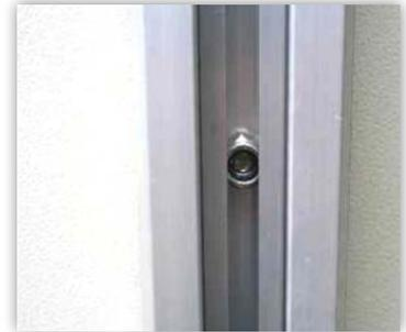
4. Slide your hand with bolt and washer between the mattress and the frame at the tent's hinge, and insert bolt into the through-hole of the frame. Secure with the nut inside the extrusion using included wrench (tighten to 4 ft-lbs). Repeat for the other three holes.
