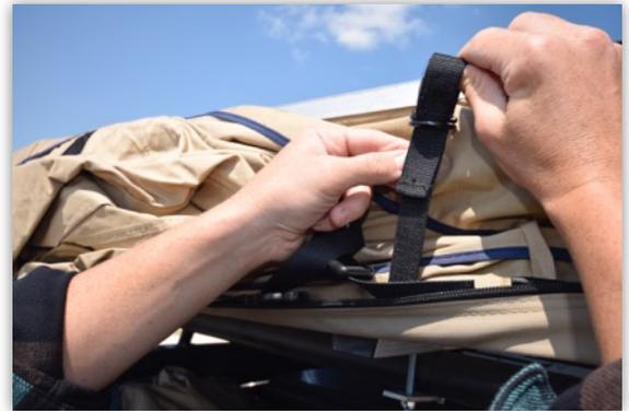
3. Undo ladder strap. Fully extend ladder by pulling the feet until all rungs are locked into place.
