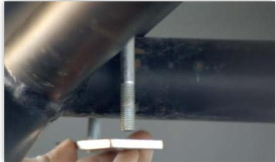
4. Slide sandwich plate under mounting rail and onto each pair of bolts, using either of the two holes on the sandwich plate that best suits the position. Tighten all eight bolts to finger tightness first, and then tighten using the 13mm end of the included wrench to 15 ft-lbs.
