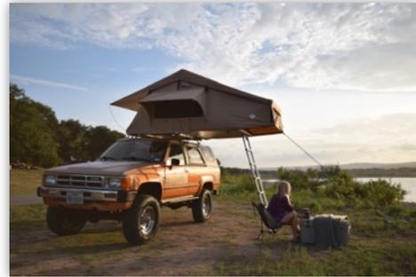
1. After verifying the static and dynamic load capacities of your rack, and that the rack is securely mounted to the vehicle, lift the tent into position, using the help of another person or a hoist. Ensure that the tent is centered on the roof rack. Mounting rails should be at least 48 inches apart.
