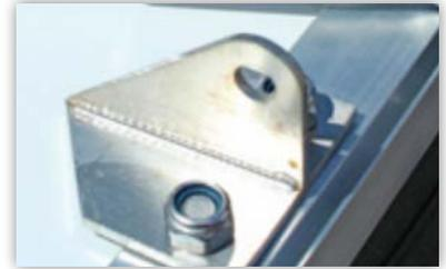
2. Unpack the ladder and place between ladder brackets, taking note to orient the ladder so that the ladder's feet are resting against the tent base. Using two washers, short bolt, nylon nut, and plastic washer, attach the ladder (see image). Tighten the ladder into position (2 ft-lbs). Cycle the ladder through its range of motion to ensure it moves freely. Finish fastening the ladder brackets to the tent frame (4 ft-lbs).
