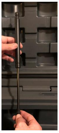
• Align the hole in the gas strut head on the stantion side with the ball stud on the lower gas strut mount and press in until it clicks into place.
