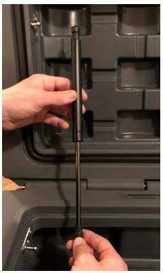
• Align the hole in the gas strut head on the stantion side with the ball stud on the lower gas strut mount and press in until it clicks into place.
