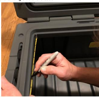
• Align the strut mount such that the long flat side is flush with the top edge of the innermost lip and aligned with the mark you just made at 8.25" and mark the center hole position.
