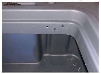
• Using your pop rivet gun. Secure the strut mount bracket using 3 of the included rivets
