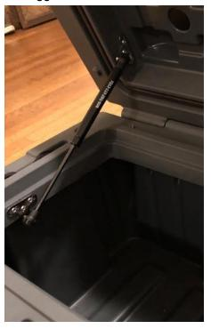
• Cycle the lid once to ensure that you installed the gas strut correctly.
