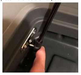
• Repeat the same thing for the top mount. You may have to adjust the position of the lid to line up the gas strut with the ball stud.
