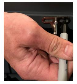
Remove the bracket and drill two more holes where you just marked
