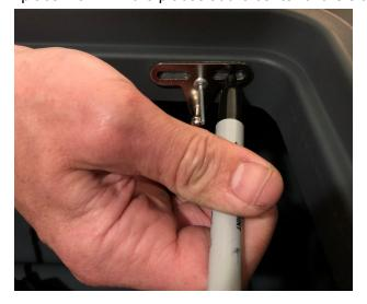
Remove the bracket and drill two more holes where you just marked
