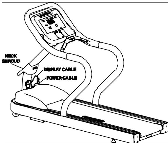
Slide the neck shroud up to gain access to the display cable. Connect the display cable to the base assembly power cord.
