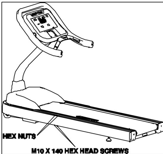
**NOTE:** Both handrails are installed in a similar manner.
