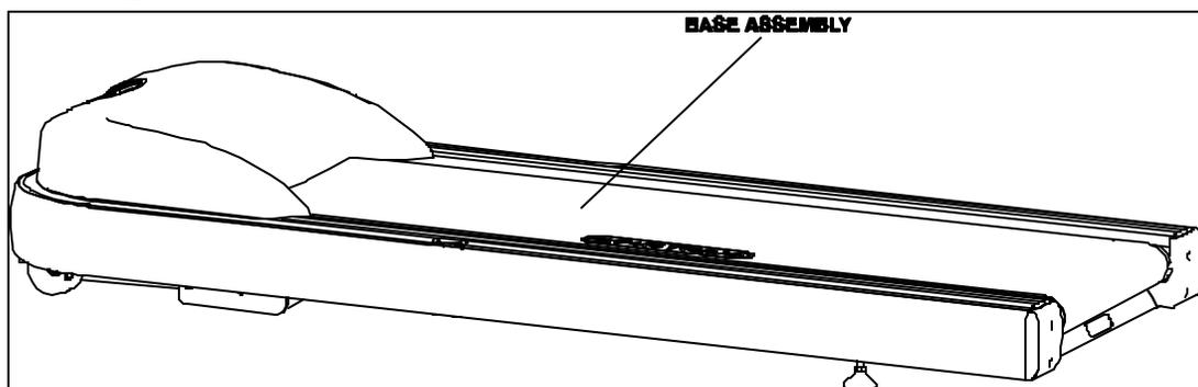
Remove all packaging material so the base assembly is sitting on the shipping crate platform. With a helper, lift the base assembly from the shipping crate platform, and place it in the location where it will be used. Be sure the selected location is level, and close to a power outlet.
