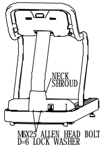
Slide the neck shroud down into position on the base assembly shroud. Secure the neck shroud to the base assembly using two M6 X 25 Allen head bolts and D=6 lockwashers.
