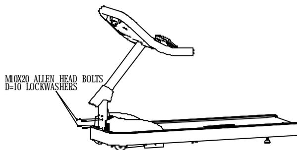
Slide the neck shroud down into position on the base assembly shroud to cover the display cable.
